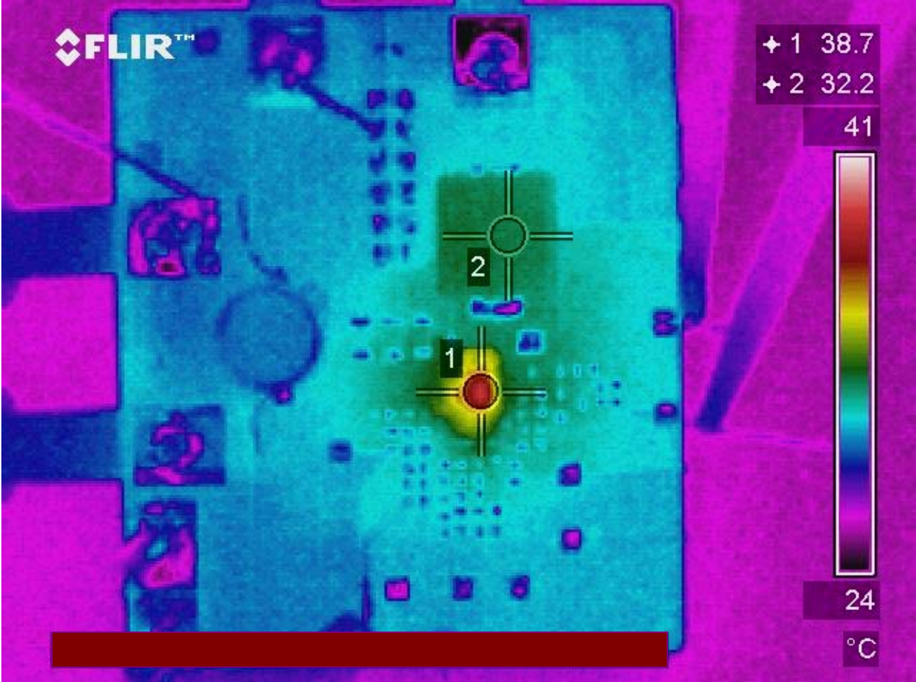
Fig.19: Thermal Image at 4A load Test Point 1: IR3832W, Test Point 2: Inductor
