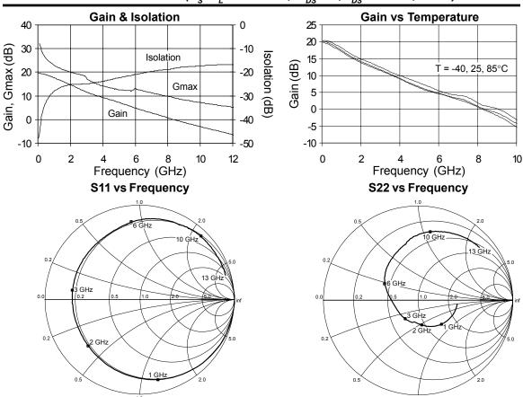
Note: S-parameters are de-embedded to the device leads with  $Z_s = Z_t = 50\Omega$ . The data represents typical performace of the device. De-embedded s-parameters can be downloaded from our website (www.sirenza.com).
