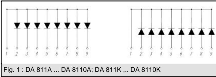
Fig. 1 : DA 811A ... DA 8110A; DA 811K ... DA 8110K
