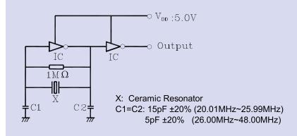
Parts shall be measured under a condition (Temp.: 20±15°C, Humidity: 65±20% R.H.) unless the standard condition (Temp: 25±3°C, Humidity: 65±10% R.H.) is regulated to measure
