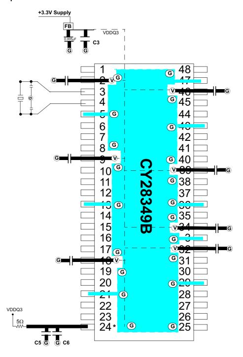
G = VIA to GND plane layer V =VIA to respective supply plane layer
