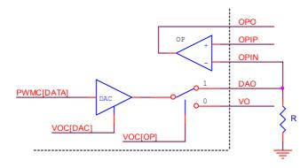
The DAC is enabled by DAC bit of VOC register. Please note that the DAC bit of VOC register will be automatically cleared when the system enter Idle or Sleep mode. So it needs to be set again when returning to Normal mode.
