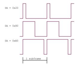
The PWM bit of VOC register controls register to enable the circuit and output driver. When PWM bit of VOC is '0', PWME bit and output drivers settings are both cleared. To use PWM for voice output, PWM bit has to be set to '1' first, then set PWME bit and enable output driver by setting the driver number. If PWM bit is disabled and enabled again, the setting for driver and PWME bit will be clear.
