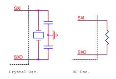
With two clock sources available, the system can switch among operation modes of Fast, Slow, Idle, and Sleep modes by the setting of OP1 and OP2 registers as shown in tables below to suit the needs of application such as power saving, etc.
