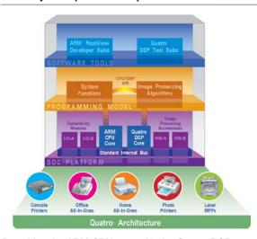
By pairing the ARM CPU core with the Quatro DSP core, the Quatro architecture provides OEMs with a unique combination of high performance processing and easy-to-use programmability. The ARM CPU core, the established leader in embedded CPU cores, delivers high performance system and control processing with dense code size and a highly regarded software development tool suite.
