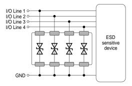
Note: Protection of I/O lines with CeraDiode array.
