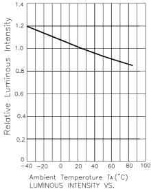
LUMINOUS INTENSITY VS. AMBIENT TEMPERATURE
