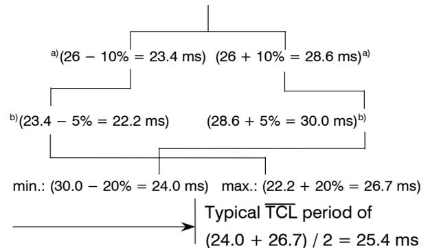
The ratio between  $T_{WD} = 26$  ms and the ( $\overline{TCL}$  period) = 25.4 ms is 0.975.
