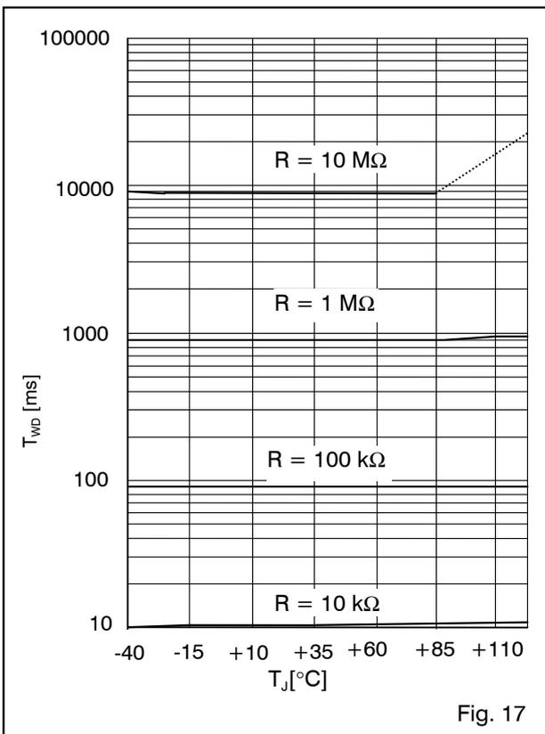
**$T_{WD}$  versus  $R$  at  $V_{OUTPUT} = 5\text{ V}$**
