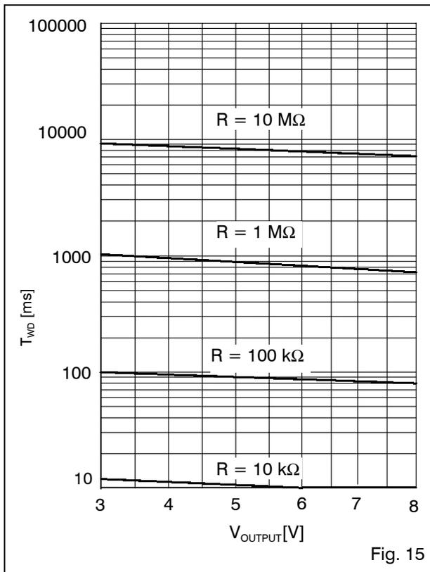
**$T_{WD}$  versus  $V_{OUTPUT}$  at  $T_J = 125\text{ }^\circ\text{C}$**
