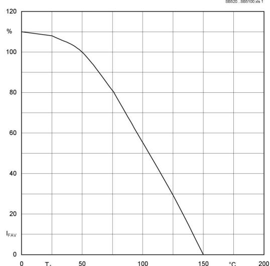
Fig. 2 Rated forward current vs. ambient temperature <sup>1)</sup>
