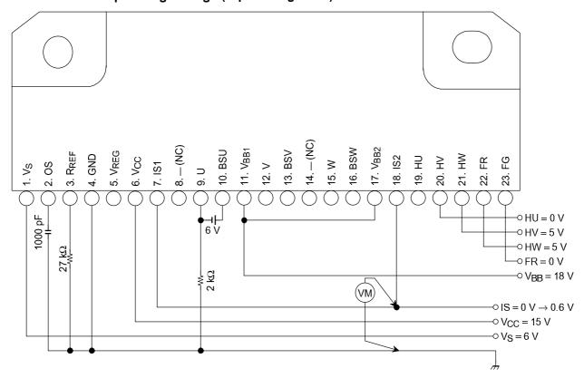
\*: Sweeps the IS pin voltage to increase and monitors the U pin voltage.
