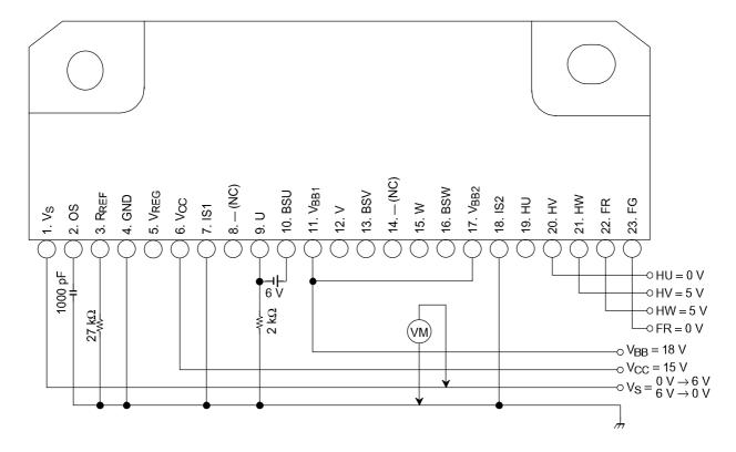
\*: Sweeps the VS pin voltage to increase and monitors the U pin.
