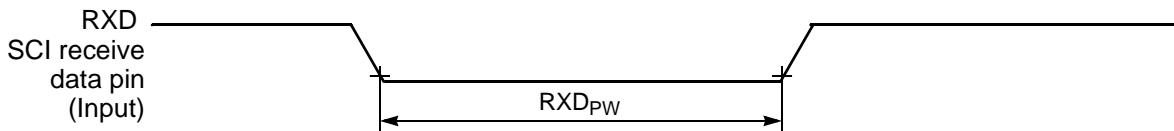
Figure 10-15 RXD Pulse Width
