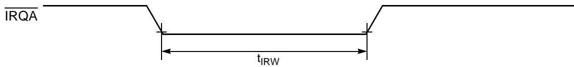
Figure 10-6 External Interrupt Timing (Negative Edge-Sensitive)
