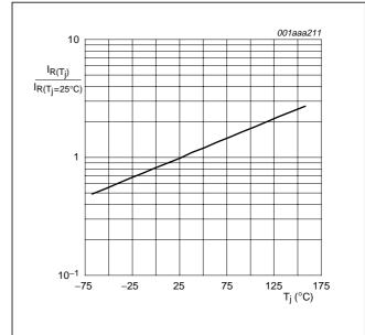
Relative variation of reverse leakage current as a function of junction temperature; typical values.
