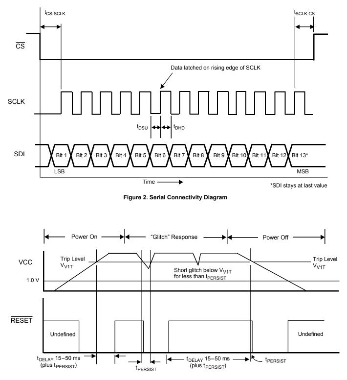
Figure 3. RESET Generation Timing Diagram (Assumes V<sub>VB+</sub> > V<sub>VB+T+</sub> During Entire Period)
