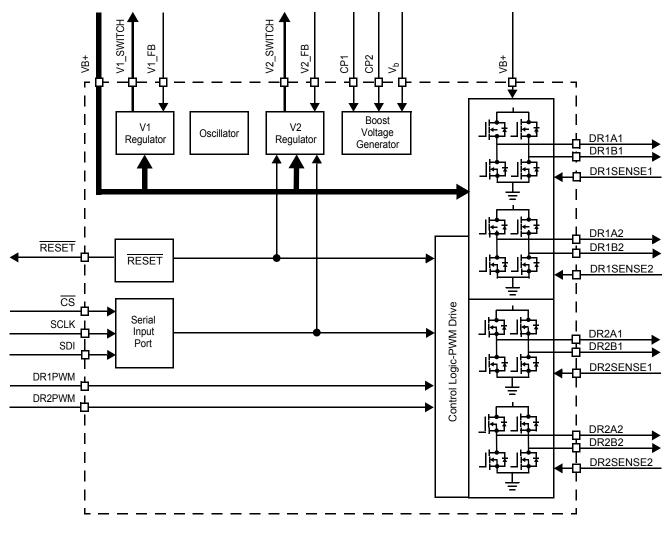
Figure 1. 34920 Simplified Internal Block Diagram
