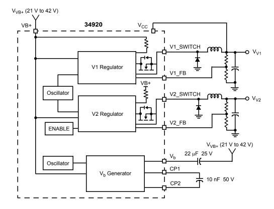
Figure 7. Voltage Regulator Functions
