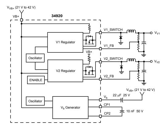
Figure 4. Voltage Regulator Functions
