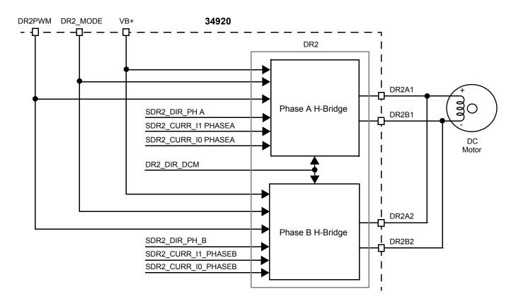
Figure 6. Simplified DC Application Diagram Showing 1 of 2 Motor Drive Circuits
