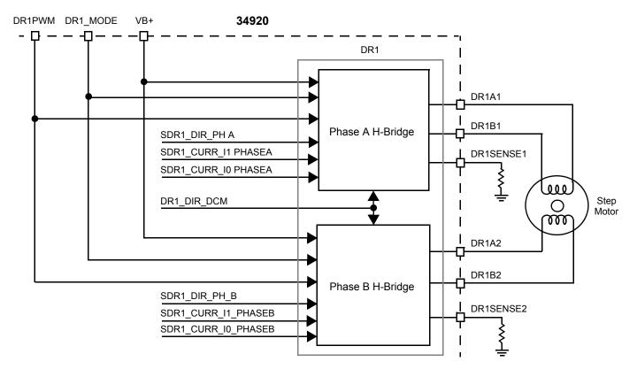
Figure 5. Simplified Step Application Diagram Showing 1 of 2 Step Drive Circuits
