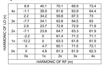
The spurious table shows the spurious signals resulting from the mixing of the RF and LO input signals, assuming down conversion. Mixing products are indicated by the number of dB below the conversion loss. The lower frequency mixing term is shown for two different RF input levels. The top number is for an RF input power of -5 dBm, the lower number is for -15 dBm.
