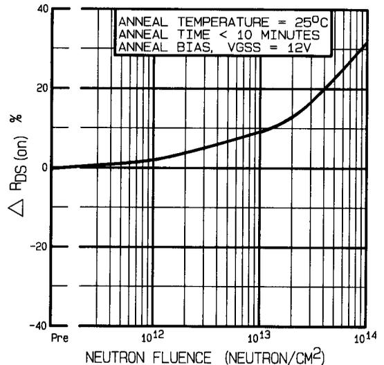
**Fig 6.** Typical On-State Resistance Vs. Neutron Fluence Level
