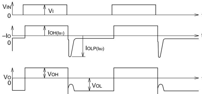
**Note:**  $I_{OH}$  and  $I_{OLP}$  correspond to base forward current  $I_{B1}$  and base reverse current  $I_{B2}$  of the transistor module to be driven respectively.
