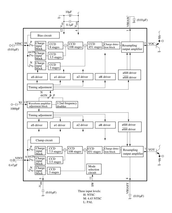
Note: When an electlytic capacitor is attached to pin 5, connect the negative pole to pin 5.
