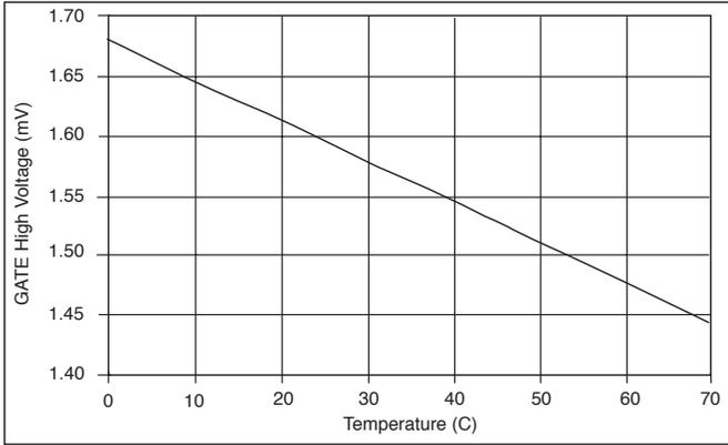
Figure 43: GATE High Voltage (100mA) vs Temperature.
