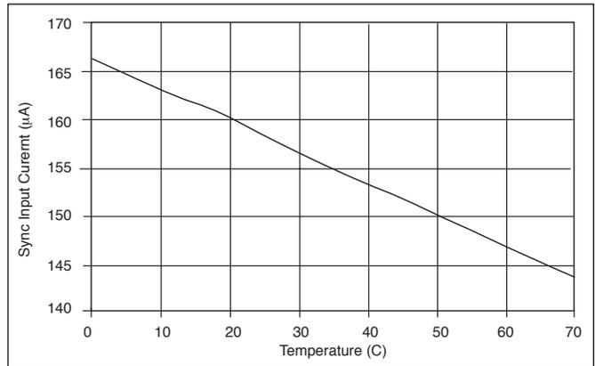
Figure 29: SYNC Input Current vs Temperature ( $V_{\text{SYNC}} = 2.4\text{V}$ ).
