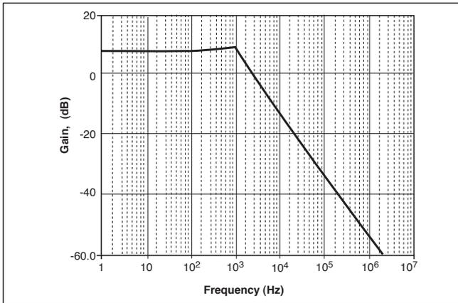
Figure 7: Bode plot of gain response for  $V_{OUT}/V_{CONTROL}$ .
