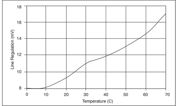
Figure 22: Line Regulation vs Temperature 9V to 20V.
