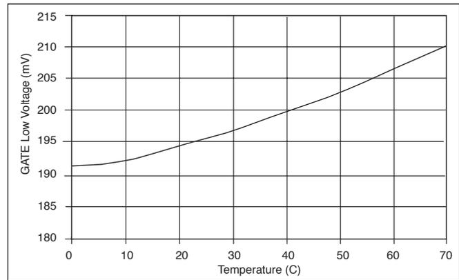
Figure 42: GATE Low Voltage (100mA) vs Temperature.
