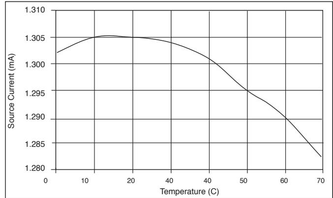
Figure 35: Error Amplifier Source Current vs Temperature.
