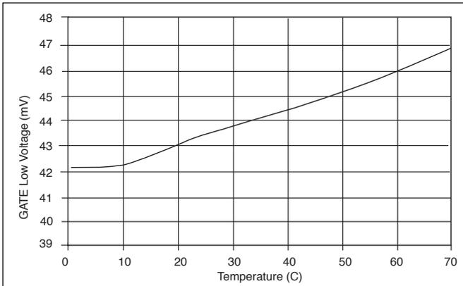
Figure 44: GATE low voltage (20mA) vs Temperature.
