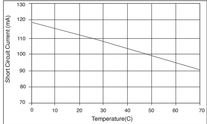
Figure 23:  $V_{REF}$  Short Circuit Current vs Temperature.
