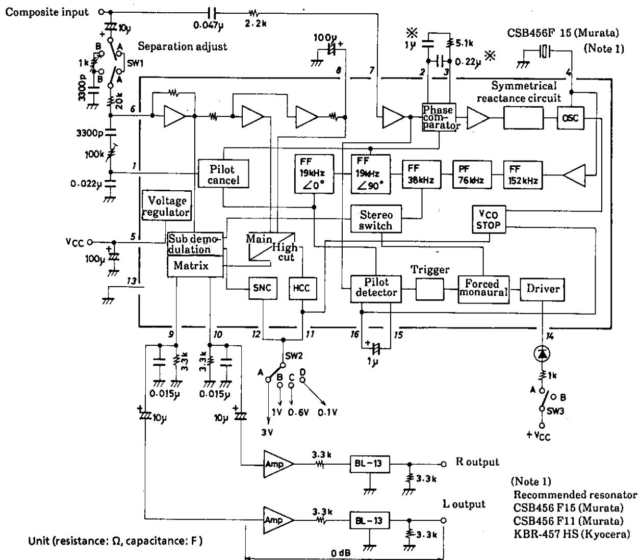
\* : When a polarized electrolytic capacitor is used in your application, the positive pole may be connected to either pin 2 or pin 3.
