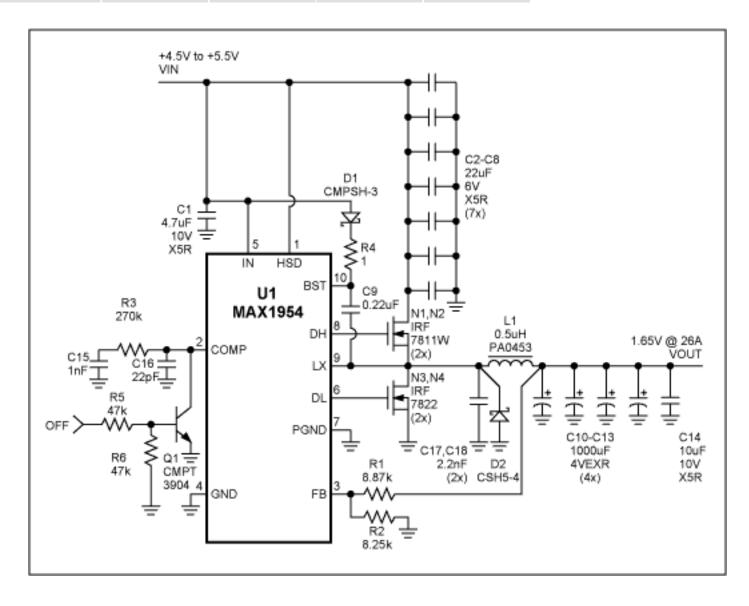
The MAX1954 Bill of Materials: 4.5V to 5.5V Input, 1.65V @ 26A Output
